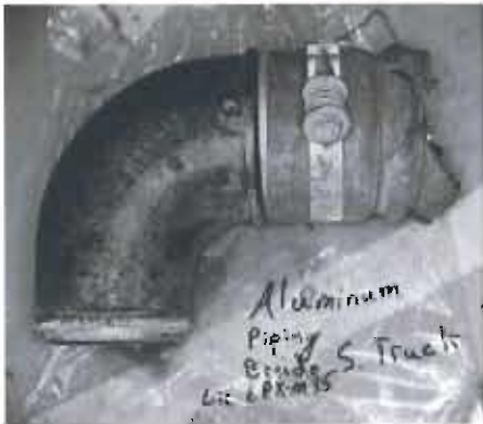
Figure 15. South truck diesel engine turbocharger discharge elbow.
