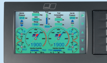
Colour display* 7'' Indication twin engine plant
